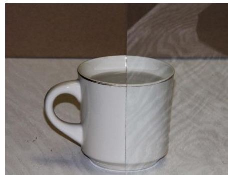
Figure 2.A. White light view of soda lime glass plate blocking ~1/2 of coffee cup.
